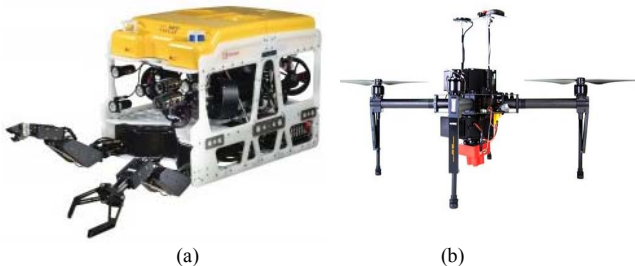
Figure 1. (a) Inspection ROV for subsea oil and gas assets ( http://www.rov.org ) (b) Inspection drones for wind turbine nacelle components ( www.aerialmediascotland.co.uk ).
